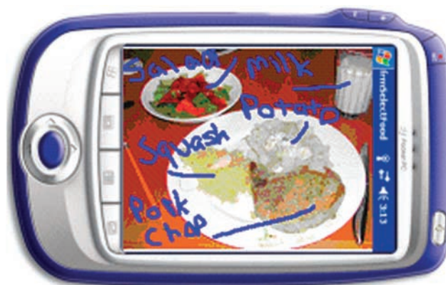
Figure 1 Input technique of using stylus to handwrite notes to label food items on a digital image of a meal.
