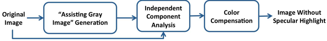
Fig. 2. Block diagram of our proposed method for specular highlight removal.
